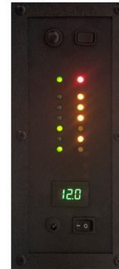
The LED control panel continuously shows the status of the system so you always know if a backflush cycle is underway, and that the system is functioning normally.
